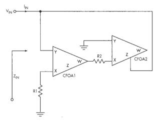
Just two current-feedback op amps and two resistors are needed to create a synthetic inductor that eliminates the drawbacks of other active-element inductors.
